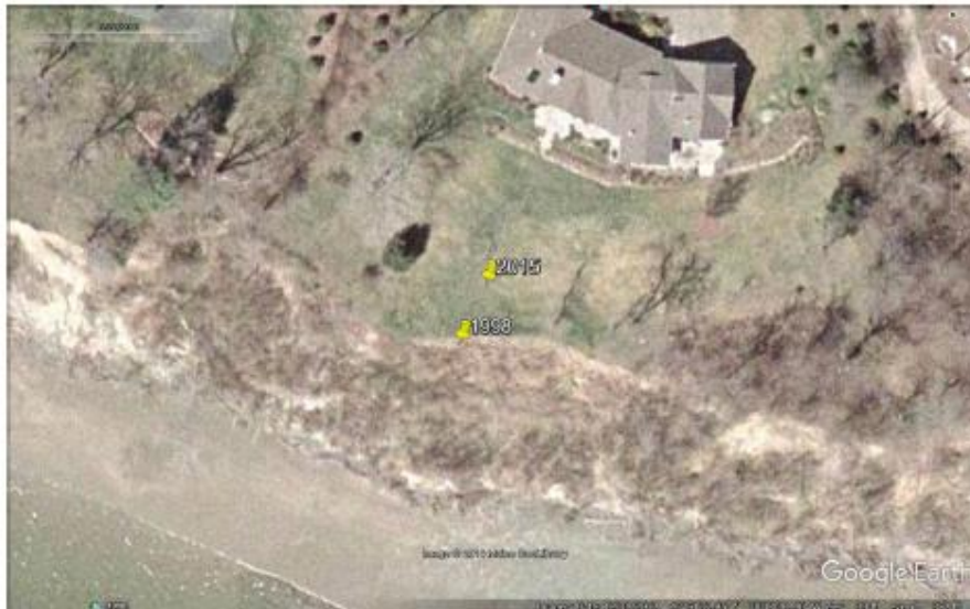
Figure 2. This December 31, 2002 photo shows the same pins as in Figure 1. From 1998 to the date of the photo there is very little retreat of the top of the bluff where the pins are located. Exposed sediment on the bluff face on the left and right sides of the photo are from slope failures that have removed vegetation. Note there are fallen trees at the base of the bluff but no patches of fringing salt marsh.
