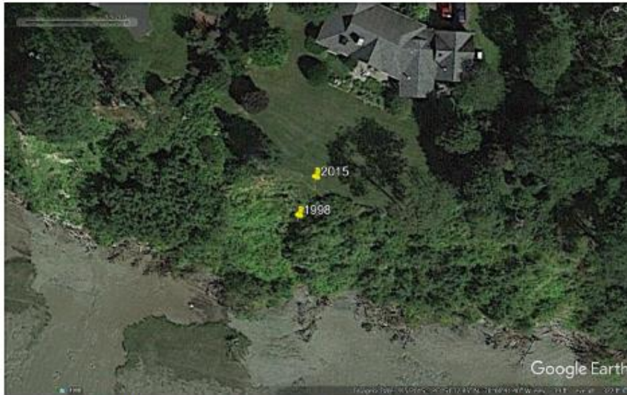
Figure 1. Shoreline change at Bunganuc Bluff seaward of the Carey residence. Each pin shows the location of the top of the bluff in different years. The bluff retreated 25 feet from 1998 to 2015 for an erosion rate of about 1.5 feet per year.
