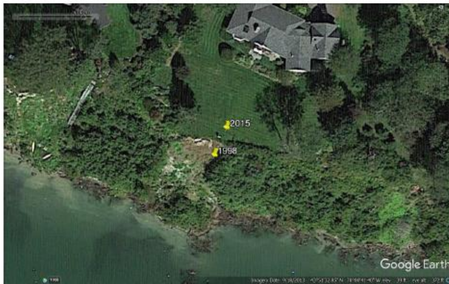
Figure 3. This September 18, 2013 image also shows the same two pins as in Figures 1 and 2 for reference. A landslide next to the 1998 pin shows vegetation and sediment slumped seaward of the base of the former bluff toe. The slump resulted in the headwall retreating 10 feet or more toward the house. The tide is relatively high and covers a fringing salt marsh seaward of the slump.
