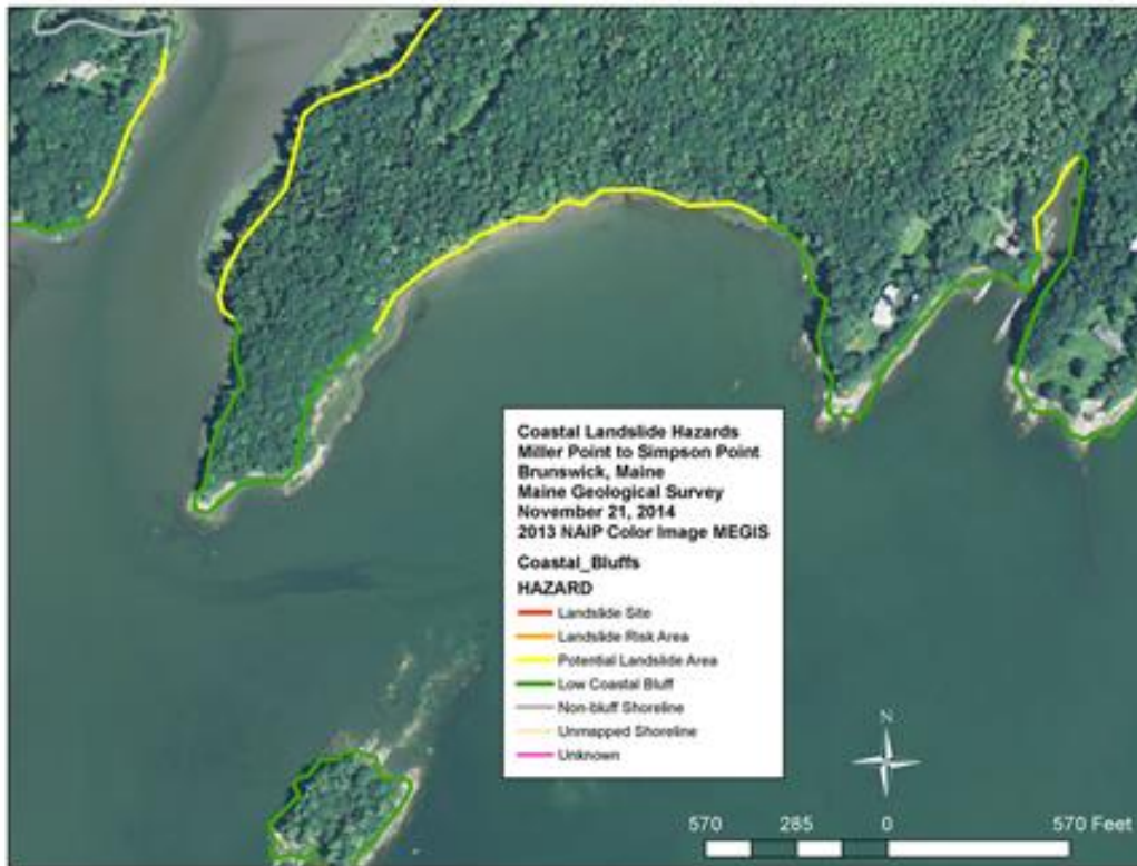
Figure 2. A portion of the MGS Coastal Landslide Hazards Map for Miller Point, Brunswick, Maine. For a full explanation of the map units and processes see Dickson (2001). The proposed hybrid shoreline stabilization project is in the Potential Landslide Area above the legend. Also visible are fringing salt marshes along the Low Coastal Bluff near both bedrock peninsulas framing the cove. Within the project area there are intermittent patches of fringing salt marsh. The tide in this image is close to high. Most of the cove (above the legend box) becomes subaerial at low tide. The engineering footprint is approximately twice the yellow line width. Map by S.M. Dickson, November 21, 2014.
