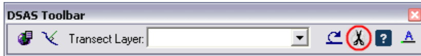
Figure 34. Screenshot of the DSAS toolbar with the Clip to Shoreline Change Envelope button circled.
