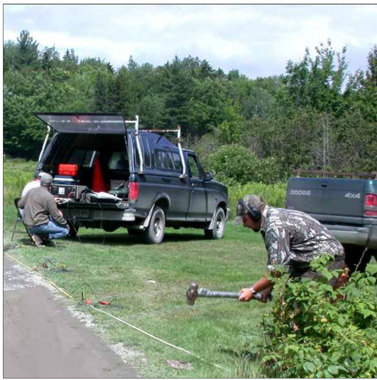
Operating a twelve-channel seismograph, Piscataquis County, Maine.
